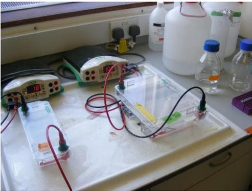
**Gel electrophoresis machinery.** Used in the lab primarily to separate DNA and/or RNA fragments by size.
