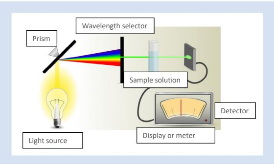
Many molecules absorb light at certain wavelengths and so by shining a beam of light through a sample and measuring how much of the beam comes out the other end, we can calculate the amount of that type of molecule there is in a sample. This can be used to measure the concentration of molecules, the rates of reaction and the way that molecules change under different conditions.
