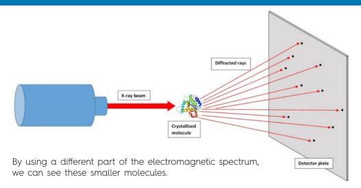
One way to do this is to turn the molecules into crystals and then fire X-rays at them. This, unsurprisingly, is known as X-ray crystallography. The image we see is a sort of shadow caused by the molecules; this is called a diffraction pattern. By using maths, we can work out what shape the molecules must be to cause that sort of pattern.
